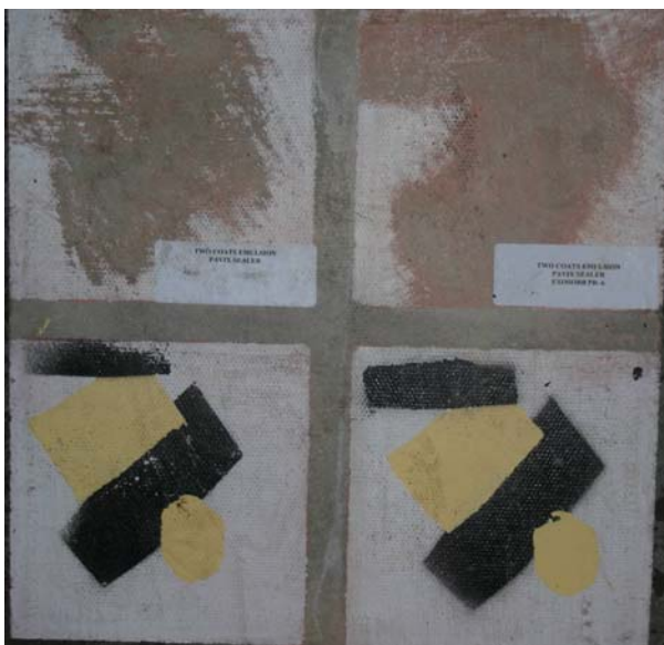
Panel 7. LHS: Emulsion > Pavix RHS: Emulsion > Pavix > Ekosorb PR A
