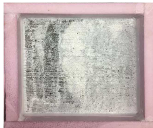
Sample with Pavix CCC100 and Curing Compound after 70 cycles of Freezing and Thawing
