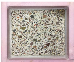
Control Sample without Pavix CCC100 and Curing Compound after 70 cycles of Freezing and Thawing
